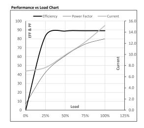
Motor Speed Torque Data Load Point P-Up BD Rated NL r/min 0 143 869 976 1000 Speed Current 80.5 72.4 47.2 15.2 7.0 Α 1.8 2.4 Torque pu
