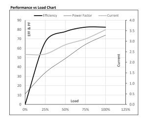
Motor Speed Torque Data P-Up BD Rated NL Load Point 0 91 782 966 1000 Speed r/min Current Α 20.9 18.8 11.7 3.5 2.4 Torque 0 pu
