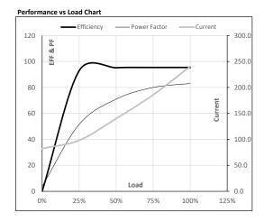
Motor Speed Torque Data LR P-Up BD Rated NL Load Point 0 143 911 990 1000 Speed r/min Current A 1299.3 1169.4 711.2 240.6 82.4 Torque pu
