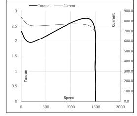
Speed r/min 0 214 1370 1489 1500 838.3 754.4 468.2 131.0 42.5 Current А 2.3 2.0 2.7 1 0 Torque pu
