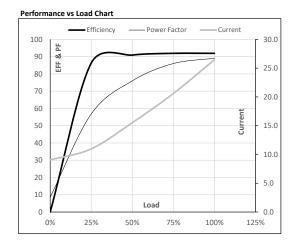
Motor Speed Torque Data P-Up BD Rated NL Load Point 600 2632 2956 3000 0 Speed r/min Current Α 222.4 200.1 130.0 26.5 9.1 Torque pu
