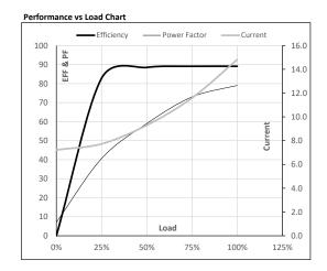
Motor Speed Torque Data LR P-Up BD Rated NL Load Point 200 868 977 1000 0 Speed r/min Current Α 81.5 73.4 47.4 14.8 7.2
