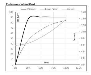
Motor Speed Torque Data LR P-Up BD Rated NL Load Point 0 300 1277 1469 1500 Speed r/min Current Α 100.3 90.3 55.1 13.7 5.8 Torque 0 pu
