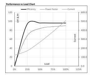
Motor Speed Torque Data P-Up BD Rated NL Load Point 214 1371 1490 1500 0 Speed r/min Current Α 3550.6 3195.5 1734.5 507.2 121.1 Torque pu
