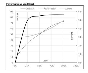
Motor Speed Torque Data LR P-Up BD Rated NL Load Point 0 91 664 958 1000 Speed r/min Current Α 29.3 26.4 19.6 5.0 3.0 Torque 0 pu
