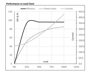
Motor Speed Torque Data LR P-Up BD Rated NL Load Point 0 200 913 992 1000 Speed r/min А 153.0 Current 2861.8 2575.6 1535.0 427.1 Torque pu
