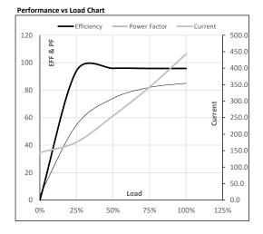
Motor Speed Torque Data Load Point P-Up BD Rated NL Speed r/min 0 200 912 991 1000 144.0 A 2703.1 2432.8 1457.9 443.1 Current 1.7 Torque pu
