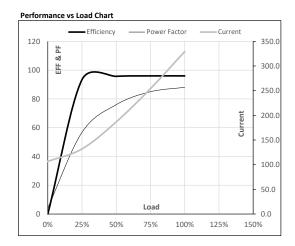
Motor Speed Torque Data LR P-Up BD Rated NL Load Point 0 300 1370 1489 1500 Speed r/min 2470.3 2223.2 1426.1 Current Α 329.4 106.7 Torque pu
