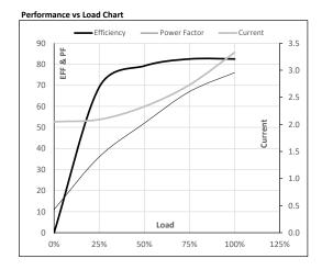
Motor Speed Torque Data LR P-Up BD Rated NL Load Point 0 91 781 965 1000 Speed r/min Current Α 19.3 17.4 10.9 3.3 2.1 Torque pu
