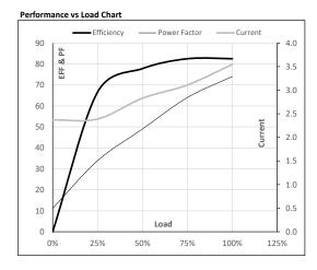
Motor Speed Torque Data LR P-Up BD Rated NL Load Point 0 91 782 966 1000 Speed r/min 3.5 Current Α 20.9 18.8 11.7 2.4 Torque pu
