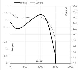
Motor Speed Torque Data Load Point LR P-Up BD Rated NL 300 0 1079 1500 Speed r/min 1450 Current 17.5 15.8 10.2 2.6 1.6 А Torque 2.9 2.4 3.4 1 0 pu
