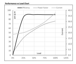
Motor Speed Torque Data LR P-Up BD Rated NL Load Point 150 680 739 750 0 Speed r/min Current Α 203.0 182.7 112.0 37.6 18.6 Torque pu
