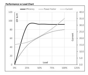
Motor Speed Torque Data LR P-Up BD Rated NL Load Point 0 143 907 986 1000 Speed r/min 35.1 Current Α 224.5 202.1 121.7 15.2 Torque pu
