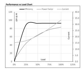
Motor Speed Torque Data LR P-Up BD Rated NL Load Point 0 214 1334 1478 1500 Speed r/min Current Α 247.8 223.0 143.4 33.5 15.1 Torque pu
