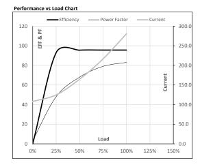
Motor Speed Torque Data LR P-Up BD Rated NL Load Point 0 91 913 992 1000 Speed r/min Α Current 1851.5 1666.4 1003.0 280.5 107.9 Torque pu
