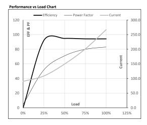
Motor Speed Torque Data LR P-Up BD Rated NL Load Point 0 150 683 742 750 r/min Speed Current A 1574.8 1417.3 852.0 266.9 90.2 Torque pu
