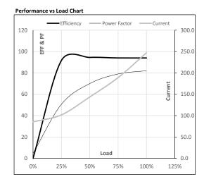
Motor Speed Torque Data Load Point P-Up BD Rated NL Speed r/min 107 683 750 A 1483.1 1334.8 791.0 247.2 85.4 Current 1.3 2.4 Torque pu
