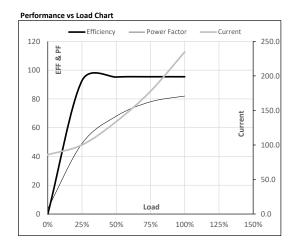
Motor Speed Torque Data LR P-Up BD Rated NL Load Point 0 143 912 991 1000 Speed r/min Current A 1338.1 1204.3 727.3 234.8 85.8 Torque pu
