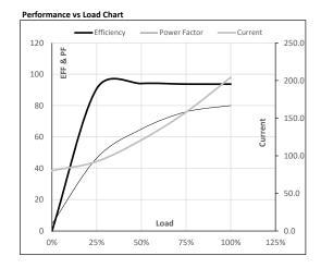
Motor Speed Torque Data LR P-Up BD Rated NL Load Point 0 150 684 743 750 r/min Speed Current A 1245.4 1120.8 681.3 204.2 80.2 Torque pu
