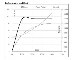
Motor Speed Torque Data LR P-Up BD Rated NL Load Point 0 143 911 990 1000 Speed r/min Current Α 863.3 777.0 473.2 162.9 61.3 Torque pu
