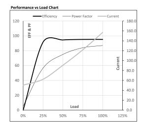
Motor Speed Torque Data Load Point P-Up BD Rated NL Speed r/min 0 300 1370 1489 1500 1003.8 903.4 546.7 156.8 50.5 Current Α 2.0 2.7 Torque pu
