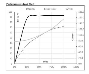
Motor Speed Torque Data LR P-Up BD Rated NL Load Point 0 150 684 743 750 Speed r/min Current Α 762.7 686.5 387.1 155.7 76.5 Torque pu
