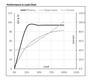
Motor Speed Torque Data Load Point P-Up BD Rated NL r/min 0 143 910 989 1000 Speed Current 630.2 567.2 346.9 101.6 40.0 Α 1.6 2.5 Torque pu
