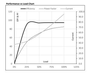
Motor Speed Torque Data LR P-Up BD Rated NL Load Point 0 214 1369 1488 1500 Speed r/min Current Α 694.7 625.2 420.5 95.2 36.9 Torque pu
