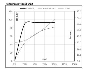
Motor Speed Torque Data LR P-Up BD Rated NL Load Point 143 908 987 1000 0 Speed r/min Current Α 464.3 417.8 259.2 67.3 29.7 Torque 2.4 pu
