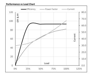
Motor Speed Torque Data LR P-Up BD Rated NL Load Point 0 143 908 987 1000 Speed r/min Current Α 464.3 417.8 259.2 67.3 29.7 Torque 2.4 pu
