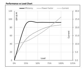
Motor Speed Torque Data LR P-Up BD Rated NL Load Point 300 0 1312 1474 1500 Speed r/min Current Α 187.1 168.4 109.0 26.3 9.9 Torque 0 pu
