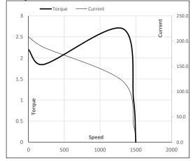
Motor Speed Torque Data P-Up BD Rated NL LR Load Point Speed r/min 0 214 1313 1469 1500 Current А 208.6 187.8 121.3 33.7 12.5 0 Torque ри 2.2 1.8 2.7 1
