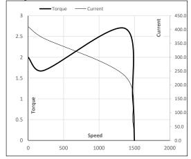
P-Up BD Rated NL LR Load Point Speed r/min 0 214 1359 1477 1500 Current А 410.6 369.5 234.6 66.2 21.1 Torque ри 2.0 1.7 2.7 1 0
