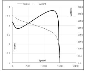
Motor Speed Torque Data P-Up BD Rated NL LR Load Point Speed r/min 0 214 1311 1471 1500 Current А 342.2 308.0 209.0 55.2 20.4 Torque ри 2.2 1.8 2.8 1 0
