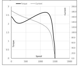
Speed r/min 0 300 1236 1465 1500 Current А 183.9 165.5 116.6 28.1 9.1 Torque pu 2.4 2.0 2.6 1 0
