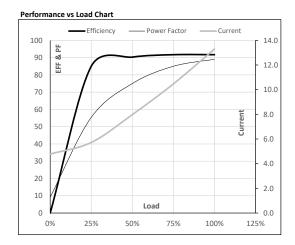
Motor Speed Torque Data LR P-Up BD Rated NL Load Point 0 600 2481 2943 3000 Speed r/min Current Α 117.0 105.3 71.2 13.3 4.8 Torque 3.1 0 pu
