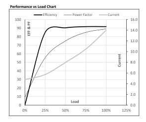
Motor Speed Torque Data LR P-Up BD Rated NL Load Point 0 600 2481 2943 3000 Speed r/min Current Α 123.2 110.9 71.2 14.0 4.8 Torque 3.1 0 pu
