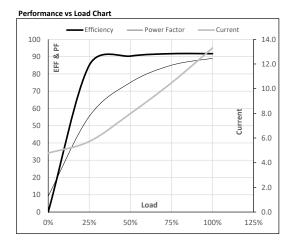
Motor Speed Torque Data LR P-Up BD Rated NL Load Point 0 600 2481 2943 3000 Speed r/min Current Α 117.0 105.3 71.2 13.3 4.8 Torque 3.1 0 pu
