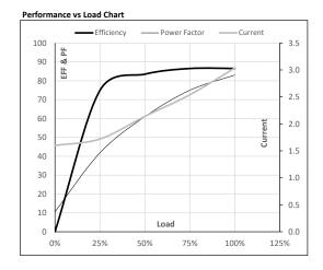
Motor Speed Torque Data LR P-Up BD Rated NL Load Point 2047 0 600 2907 3000 Speed r/min Current Α 26.4 23.8 16.4 3.0 1.6 Torque 4.4 0 pu
