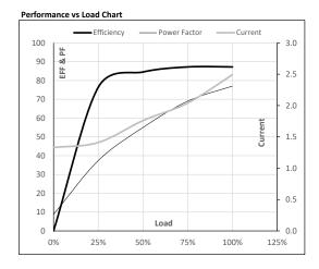
Motor Speed Torque Data LR P-Up BD Rated NL Load Point 0 300 1102 1451 1500 Speed r/min 2.5 Current Α 17.7 15.9 10.2 1.3 Torque 0 pu
