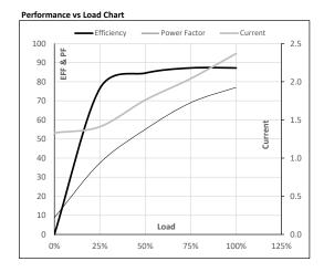
Motor Speed Torque Data LR P-Up BD Rated NL Load Point 0 300 1102 1451 1500 Speed r/min 15.1 Current Α 16.8 10.2 2.4 1.3 Torque 0 pu
