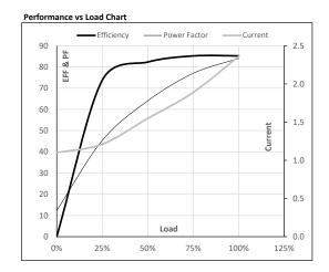
Motor Speed Torque Data LR P-Up BD Rated NL Load Point 600 1990 2891 3000 0 Speed r/min Current Α 18.4 16.6 11.5 2.4 1.1
