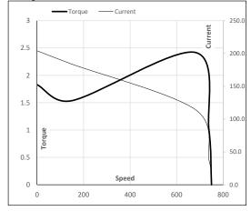
Motor Speed Torque Data P-Up BD Rated NL LR Load Point Speed r/min 0 150 680 739 750 Current А 204.2 183.8 114.7 37.8 19.0 Torque ри 1.8 1.5 2.4 1 0
