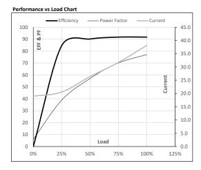
Motor Speed Torque Data LR P-Up BD Rated NL Load Point 0 150 680 739 750 Speed r/min Current Α 206.0 185.4 114.7 38.1 19.0 Torque pu
