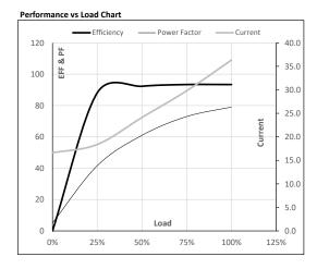
Motor Speed Torque Data LR P-Up BD Rated NL Load Point 0 200 907 986 1000 Speed r/min Current Α 236.3 212.6 130.5 36.3 16.6 Torque pu
