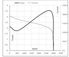
Motor Speed Torque Data P-Up BD Rated NL LR Load Point Speed r/min 0 600 2745 2984 3000 Current А 1913.1 1721.8 1217.6 269.5 87.2 Torque pu 2.1 1.8 3.5 1 0
