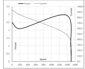
Motor Speed Torque Data P-Up BD Rated NL LR Load Point Speed r/min 0 214 1372 1491 1500 Current А 938.5 844.7 499.8 138.0 44.5 0 Torque ри 2.5 2.1 3.0 1
