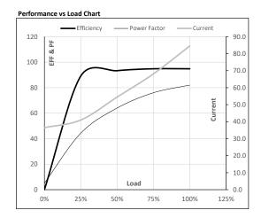
Motor Speed Torque Data LR P-Up BD Rated NL Load Point 143 912 991 1000 0 Speed r/min Current Α 600.0 540.0 324.7 84.5 36.5 Torque 0 pu
