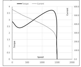
Motor Speed Torque Data P-Up BD Rated NL LR Load Point Speed r/min 0 300 1367 1486 1500 Current А 567.7 511.0 316.7 67.6 29.4 0 Torque ри 2.9 2.4 3.7 1
