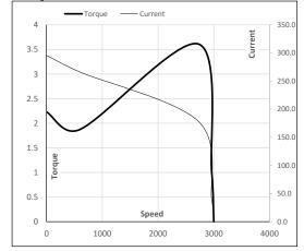
Motor Speed Torque Data P-Up BD Rated NL LR Load Point Speed r/min 0 600 2725 2963 3000 Current А 295.7 266.1 178.4 40.0 12.6 Torque ри 2.2 1.9 3.6 1 0
